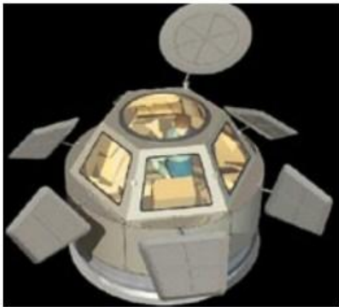
Deployed shutters for Cupola windows.
